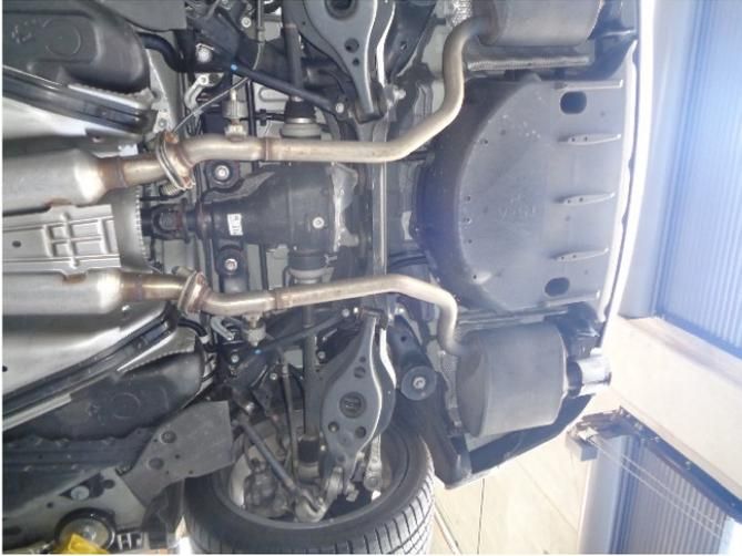
1. Remove your OEM exhaust center section by first unbolting the two tail pipe assemblies.
